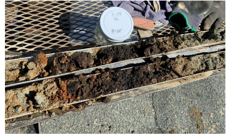
Sampling During Geotechnical Investigation CASE STUDY NO.2
